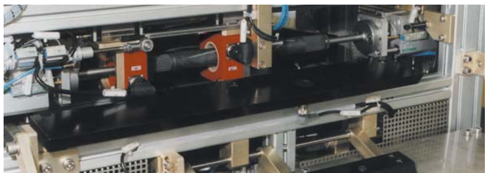
Test coils move to four test positions (indicated by arrows) over the shaft lengths.
