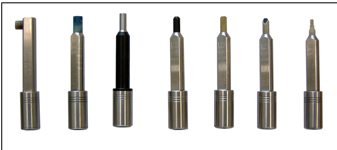
Photo 1: a variety of crack test probes
