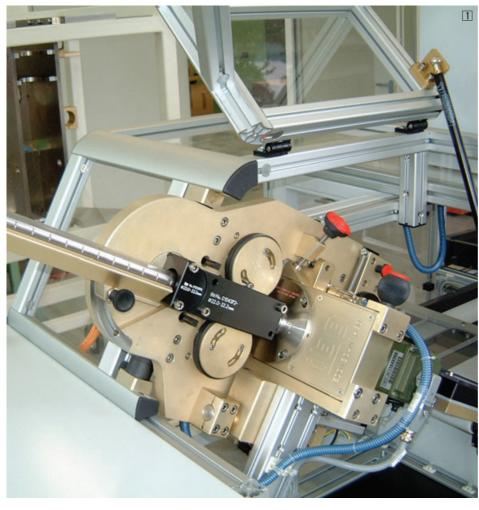
Photo 1: Rotating head eddyscan®H with test parts
