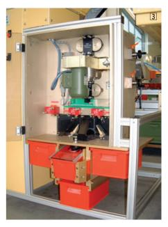
Photos 2+3: Test systems for cylinder rollers and needles
