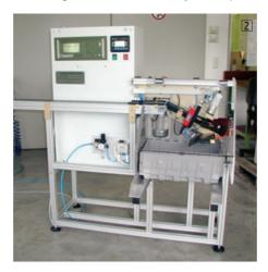
Photo 2: Semi-automatic test system for stampings
