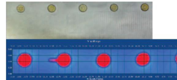
Subsurface flaw from steel fastener
