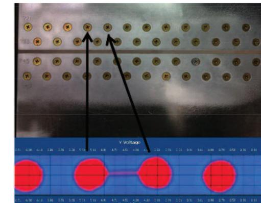
Flaw between steel fasteners
